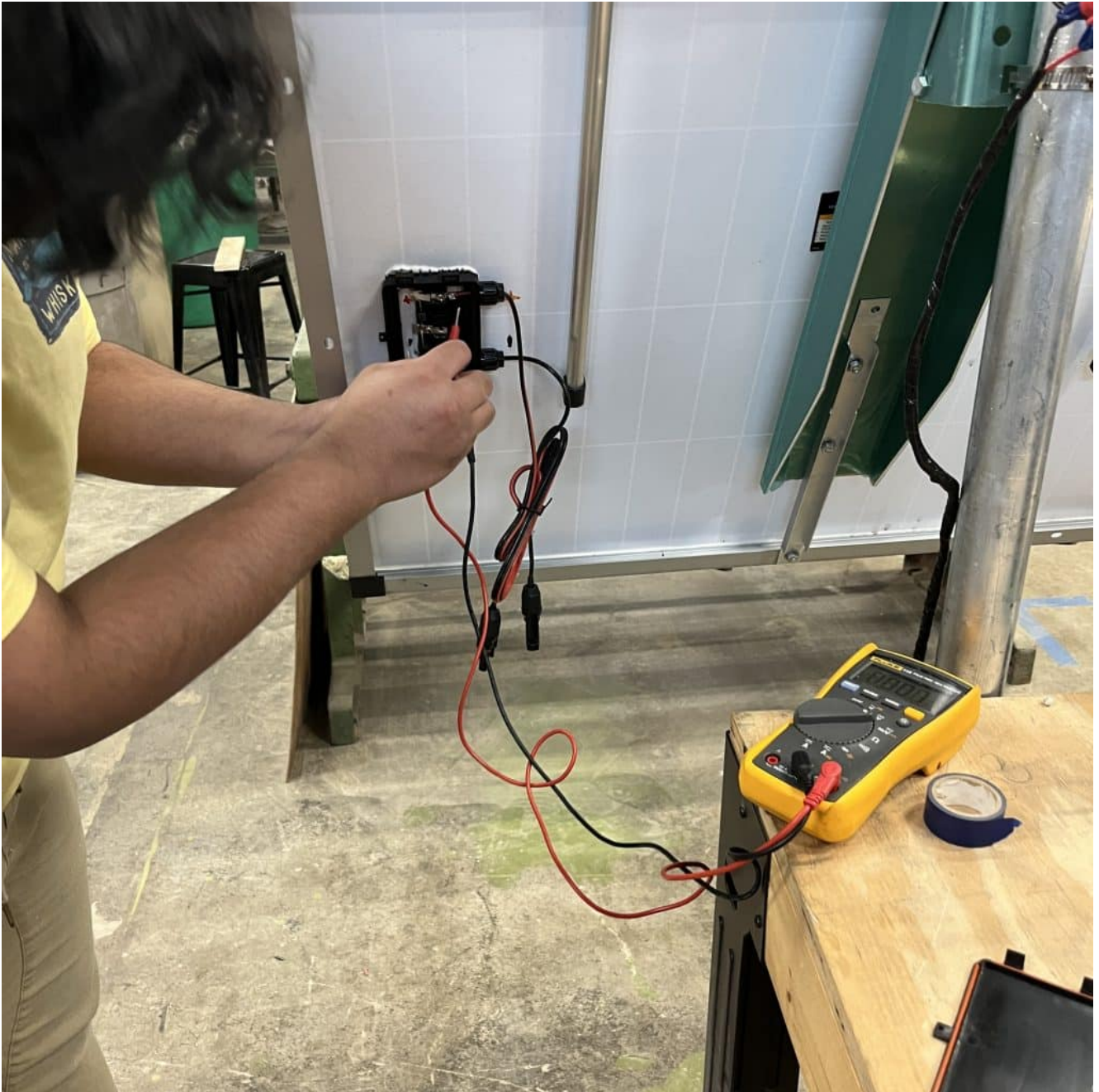
Sudman Testing the voltage of the 100W Panel
